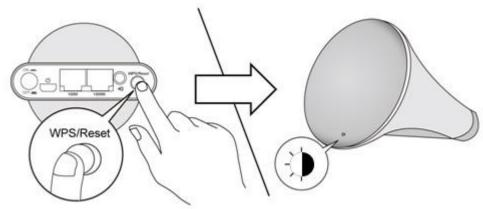
The devices will establish a connection. When a connection is successful, the bridge's LED will display on (white). If a connection is not successful, the LED will flash (red) – in this case please return to <u>II-2. WPS Setup</u> Step 1.
