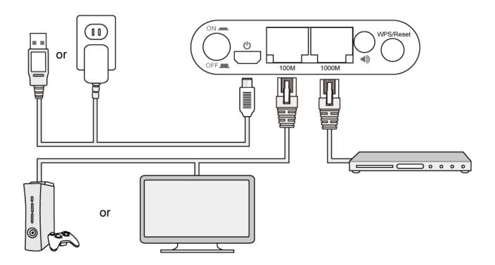
2. Connect the CV-7438nDM's power supply to a wall socket or an available USB port, and press the power on/off button to switch the device on. Ensure the LED is on (white).
