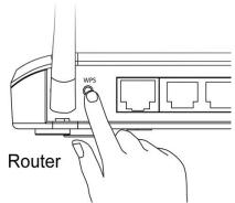
**3.** Within two minutes, press and hold the WPS button on the CV-7438nDM for\_2 seconds to activate the WPS function. The LED should flash (white) to indicate that WPS is in progress.
