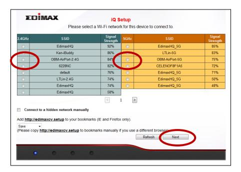
If you use a hidden network, to connect to a hidden SSID, check the "Connect to a hidden network manually" box and enter the SSID and security key information.
