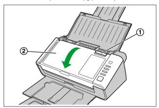
3. Clean the scanning glass area (1) and reference area (2) using a soft and dry cloth.
