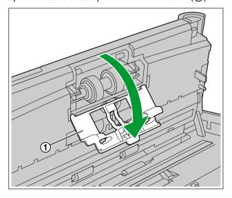
**4.** Remove the double feed prevention roller (1).
