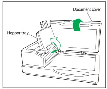
**4** Clean up the surface of flatbed glass with the roller cleaning paper (KV-SS03) to remove the dirt.
