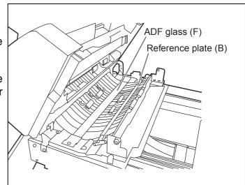
Clean the ADF glass (B) and reference plate (F) with the roller cleaning paper (KV-SS03).
