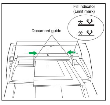
**7** Remove the document and lock the document guide. Slide the document guides selector in the direction shown in the illustration until the  $\mathbf{\nabla}$  (1) and  $\mathbf{\Theta}$  (2) marks are aligned to lock the document guide.
